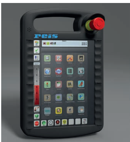
3. touch-based user interface with large control elements
