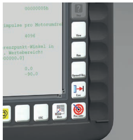
2. Housing frame with haptic marks on the edge of the housing: edges, corners, finger recesses and nubs
