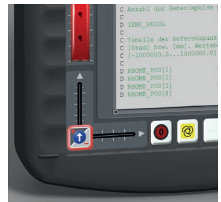
5. function selection by means of L-shaped gesture along two housing edges
