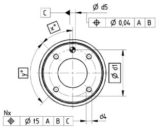
A dowel pin is required in addition to the internal or external centering to fix the position
