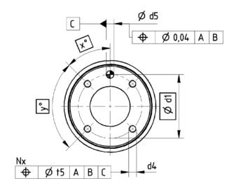
A dowel pin is required in addition to the internal or external centering to fix the position
